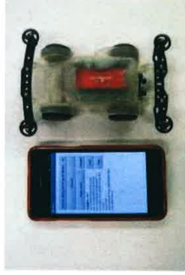
Figure 1 Device driven by application using acceleration sensor and shuffling movement
