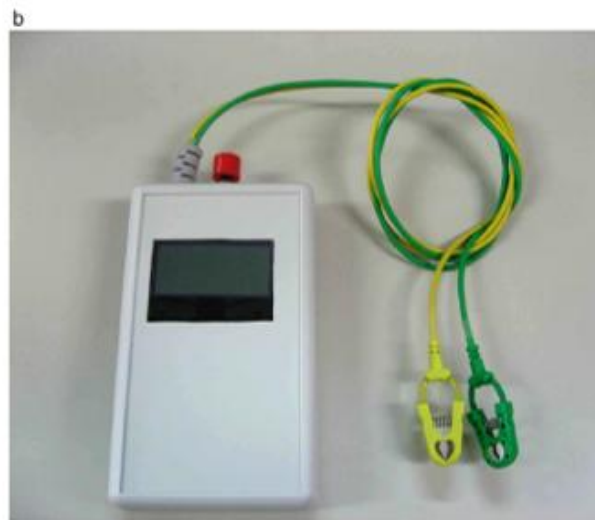
Fig. 4: Skin impedance measurements. (a) Skin impedance meter. The skin impedance values were measured using the Skin Impedance Meter Ver.3.03 made by Live Aid Co., Ltd. (b) Skin impedance electrodes. Two electrodes (Echorode III made by Fukuda Denshi Co., Ltd) were attached to the subject's left palm. An electrode clip was connected to each of the electrodes
