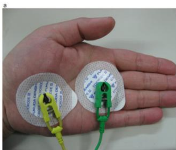
Fig. 4: Skin impedance measurements. (a) Skin impedance meter. The skin impedance values were measured using the Skin Impedance Meter Ver.3.03 made by Live Aid Co., Ltd. (b) Skin impedance electrodes. Two electrodes (Echorode III made by Fukuda Denshi Co., Ltd) were attached to the subject's left palm. An electrode clip was connected to each of the electrodes
