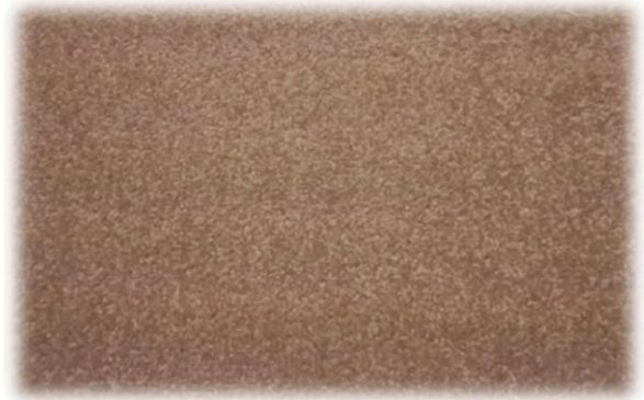
Fig. 1: Tile carpet. The carpets used were tile carpets made by TOLI Corporation. Product name: SMIFEEL ATTACK 260; pile length: 5 mm; thickness of the backing layer: 5 mm; total thickness: 10 mm; color: mocha. Product number: AK2603. 100% Nylon
